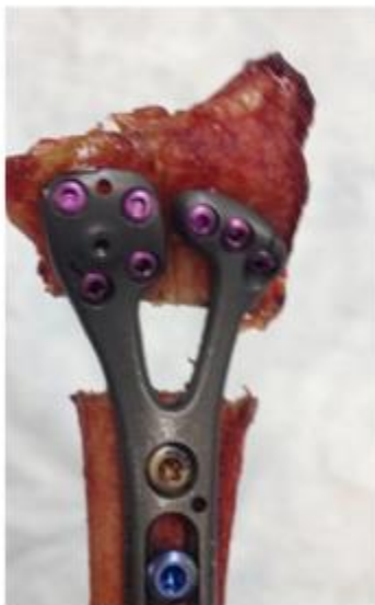
Figure 1. Specimen from Group F showing a simulated AO C-3 fracture and volar plate fixation with 7 distal screws.
